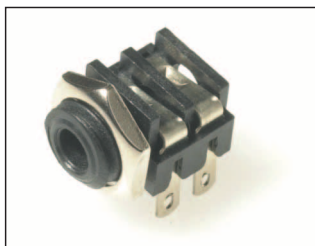
S6/BB mono switched 3.5mm Jack Socket. Panel mounting with solder tags. Also available with Special 'C' Contact to suit Far Eastern plugs.
